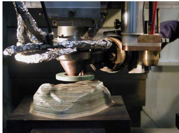
Fig. 8: High-speed generation of a tool section by induction assisted laser beam build-up welding
